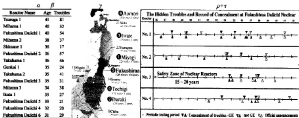
Figure 2: The empirical data underlying the 'Fukushima Decommissioning Formula', employing \alpha , \beta , \gamma , \rho , \tau . On the left is shown the age of operation and reported troubles. In the middle are shown the number of earthquakes in the Tohoku Region (from 2008.9 to 2009.8) and the locations of nuclear plants (Masai, 2009). On the right is shown a summary of the hidden troubles and record of concealment of nuclear power plant data at the Fukushima Daiichi Plant by TEPCO.
